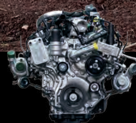
2.7L ECOBOOST 325 Max. Horsepower 400 lb.-ft. of Torque
